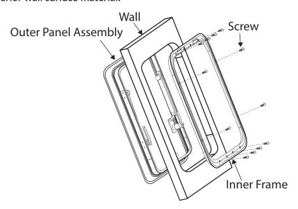
We use an inner frame ring system, which can accommodate the following wall thicknesses:
