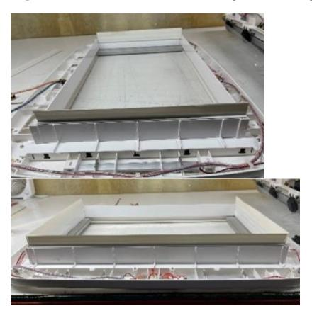
**Step 5:** Firmly press the expansion ring strips into place to ensure they are fully seated and adhered.
