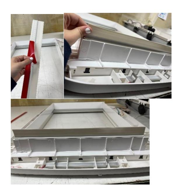
**Step 4**: Once the two short sides are installed, repeat the same steps for the two long sides.
