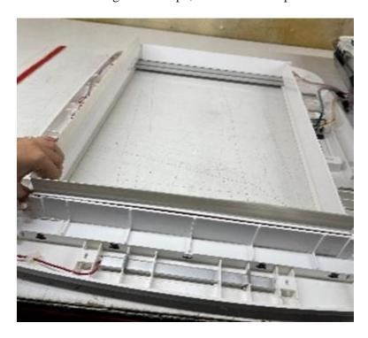
After verifying fitment, clean the mating surfaces using isopropyl alcohol.
