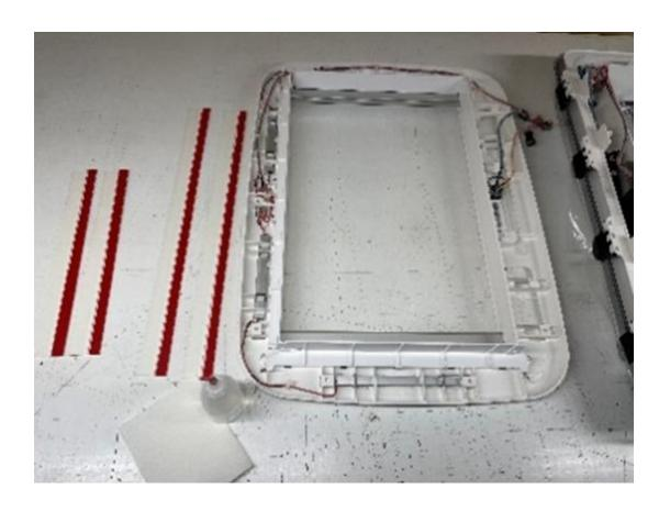
**Step 2**: Prior to removing the red tape, test fit the trim pieces.
